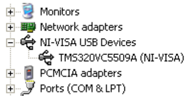
Figure 17. NI-VISA Driver Verification Using Device Manager
