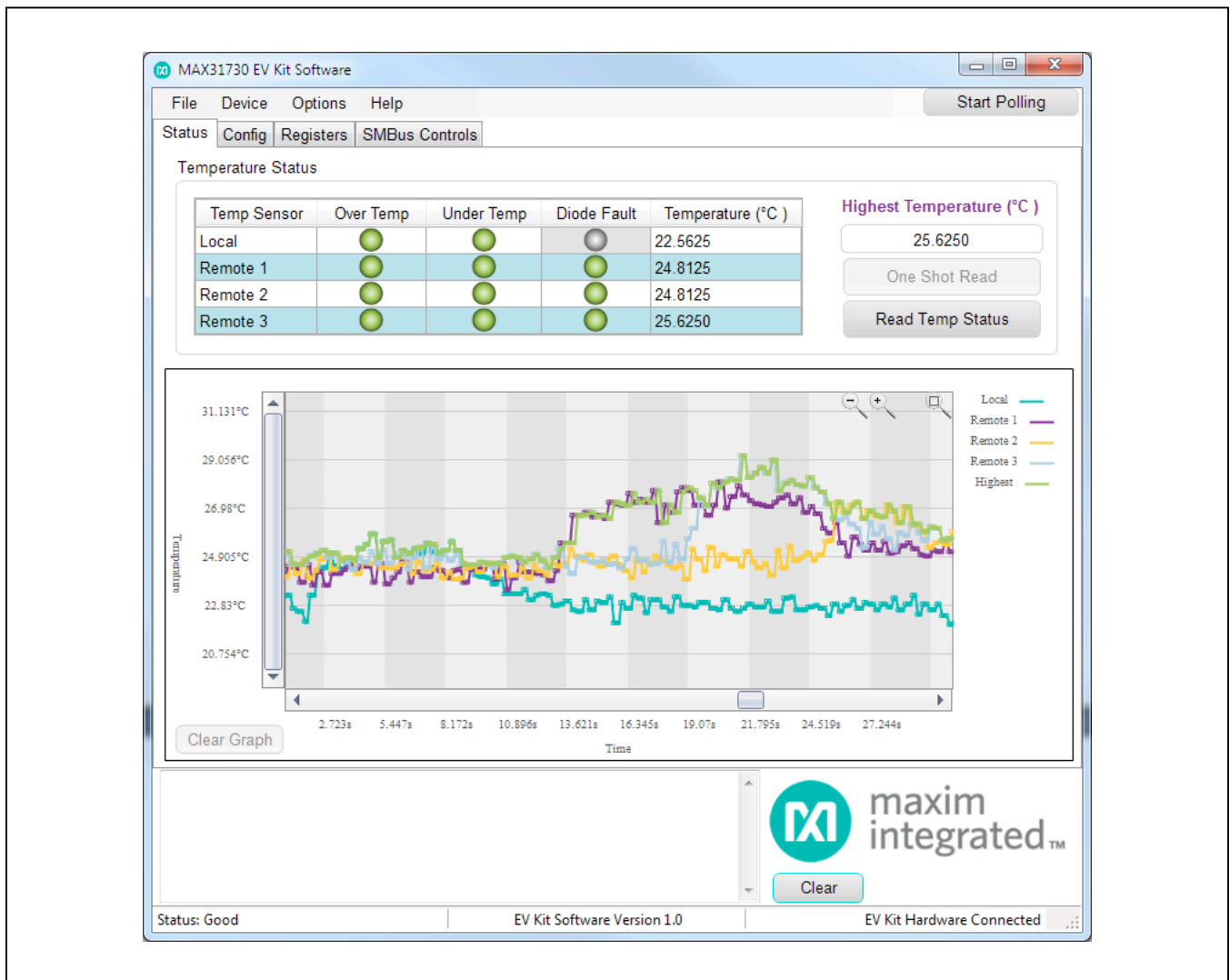
Figure 1. MAX31730 EV Kit Software GUI (Status Tab)
