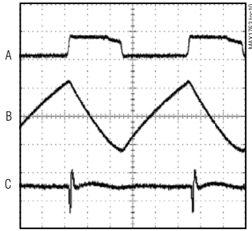
200ns/div V_{IN} = 1.1V , V_{OUT} = 3.3V , I_{OUT} = 20mA A: LX NODE, 5V/div B: INDUCTOR CURRENT, 0.1A/div, AC COUPLED C: OUTPUT RIPPLE, 0.1V/div, AC COUPLED
