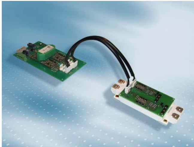
Figure 2 The 'Flexible driver Starter Kit' for EconoDual™3 module
