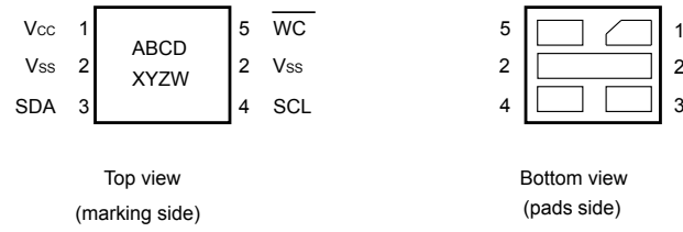
Figure 3. UFDFPN5 (DFN5) package connections
