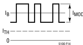
Figure 14. Components of the Laser Bias and Modulation Currents
