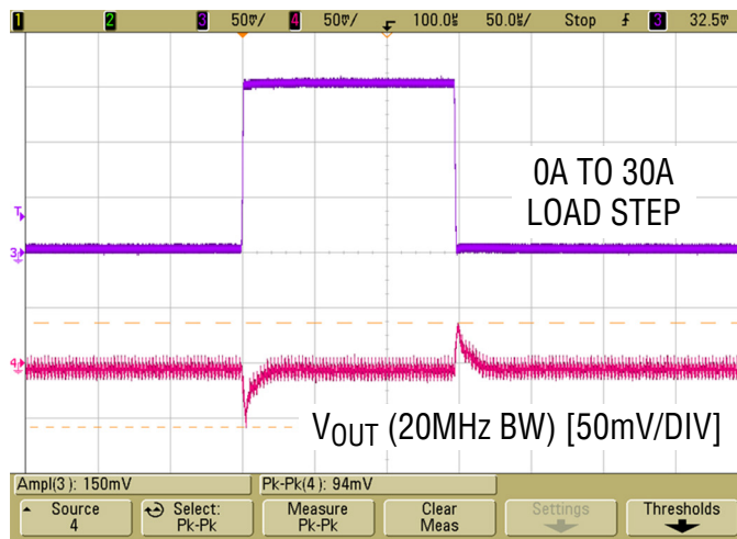
Figure 7. Transient Performance at V_{IN} = 12V , V_{OUT} = 1.0V , I_{OUT} = 0A to 30A , f_{SW} = 400kHz
