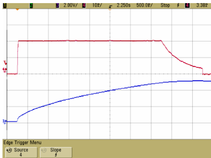
Figure 4. Charging Mode, V_{SYS} 2.5V, Input Current Set to 2.0, Ch 4 (Red) Input Current, 1.0A/DIV, Ch3 (Blue) VCAP Voltage
