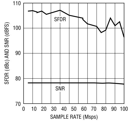
LTC2205-14: SFDR and SNR vs Sample Rate, f_{IN} = 5.1\text{MHz} , RAND = 0, DITH = 0
