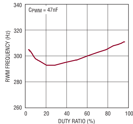
PWM Signal Generator Frequency vs Duty Ratio
