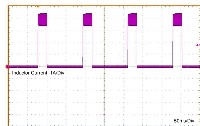
Figure 11. Inductor Current Burst in Short-Circuit Mode
