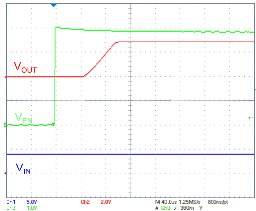
Figure 27: Enable transient ( I_{OUT} = 250 mA)
