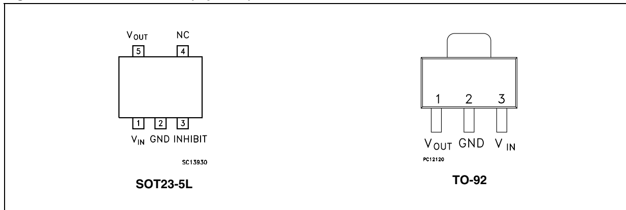
Figure 2. Pin connections (top view)
