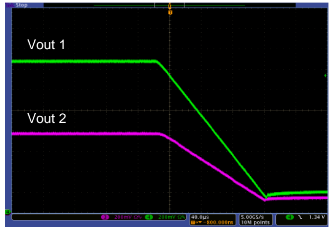
Figure 15: MPoL Tracking Shutdown
