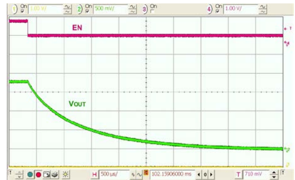
Figure 27. Shutdown, No Load, Output Discharge Enabled
