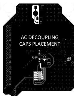
Figure 33. Example DS90UR241-Q1 EMC Layout
