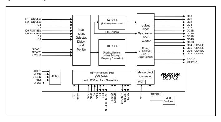
See Figure 7-1 for a detailed view of the T0 and T4 DPLLs and the Output Clock Synthesizer and Selector block.
