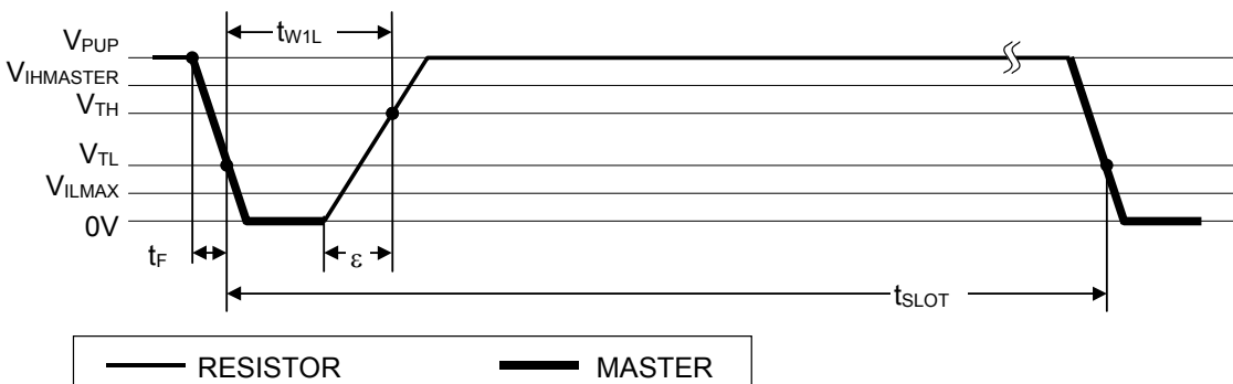
Figure 11. READ/WRITE TIMING DIAGRAM
