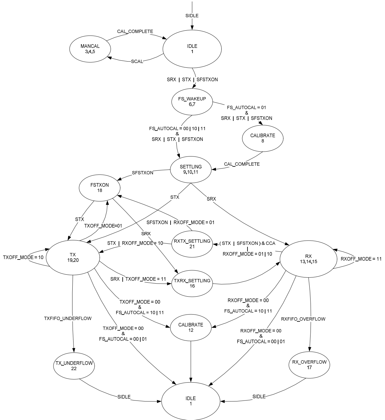
Figure 55: Complete Radio Control State Diagram
