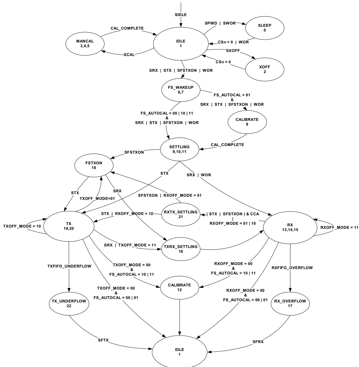
Figure 3-15. Complete Radio-Control State Diagram
