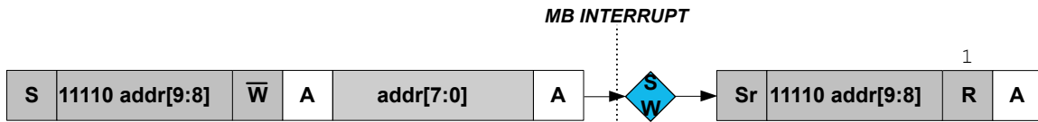
Figure 33-9. 10-bit Address Transmission for a Read Transaction
