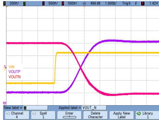
Figure 50. Step Response of the AMC1301 Device
