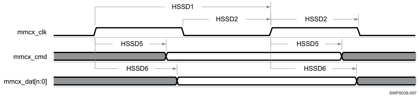
Figure 6-74. MMC2 and MMC3 Interfaces—High-Speed SDIO Mode—Data/Command Transmit (1)
