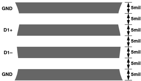
Figure 17. Arrangements of Signal Tracks
