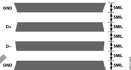
Figure 25. Arrangement of Signal Tracks
