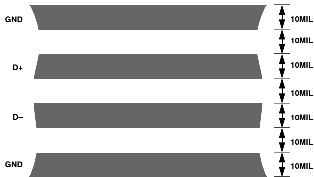
Figure 18. Typical Arrangement of Signal Tracks
