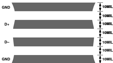
Figure 34. Arrangement of Signal Tracks
