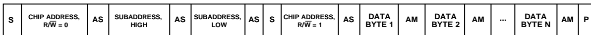
S = START BIT, P = STOP BIT, AM = ACKNOWLEDGE BY MASTER, AS = ACKNOWLEDGE BY SLAVE. SHOWS A ONE-WORD WRITE, WHERE EACH WORD HAS N BYTES.
