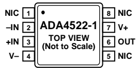
Figure 3. ADA4522-1 Pin Configuration
