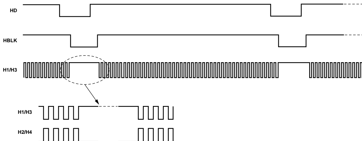
Figure 24. Horizontal Blanking (HBLK) Pulse Placement
