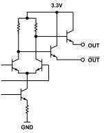
Figure 43. LVPECL Output Simplified Equivalent Circuit
