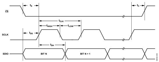
Figure 51. Serial Control Port Timing Diagram—Write
