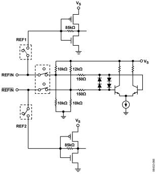
Figure 34. REFIN Equivalent Circuit
