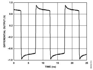
Figure 14. LVPECL Output (Differential) at 100 MHz
