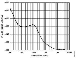
Figure 23. Phase Noise (Absolute) Clock Generation; Internal VCO at 1.97 GHz; PFD = 15.36 MHz; LBW = 143 kHz; LVPECL Output = 122.88 MHz
