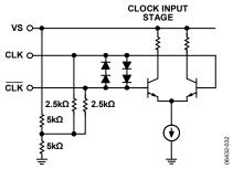
Figure 37. CLK Equivalent Input Circuit
