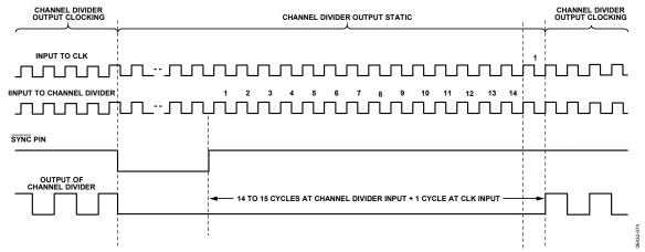
Figure 42. SYNC Timina When VCO Divider Is Not Used—CLK Input Only
