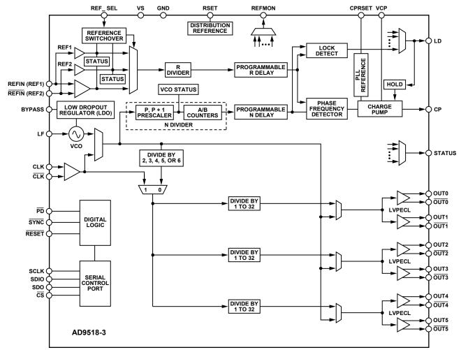
Figure 27. Detailed Block Diagram
