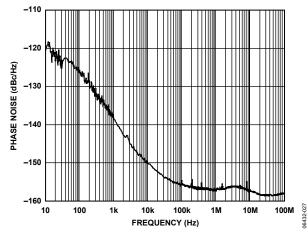
Figure 21. Phase Noise (Additive) LVPECL at 200 MHz, Divide-by-5
