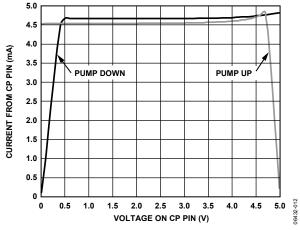
Figure 8. Charge Pump Characteristics at  $V_{CP} = 5.0 \text{ V}$
