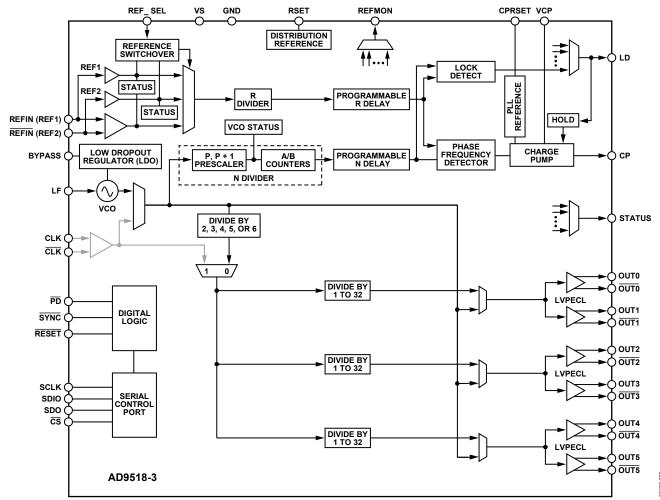
Figure 29. Internal VCO and Clock Distribution
