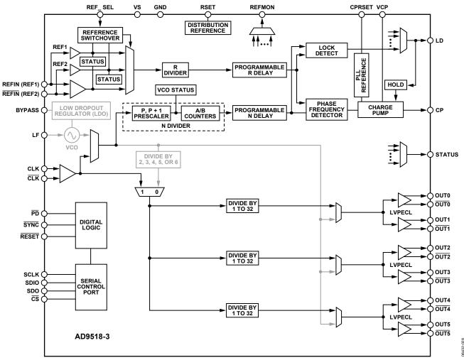
Figure 30. Clock Distribution or External VCO < 1600 MHz
