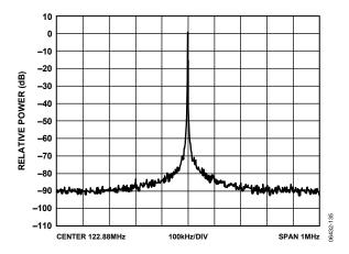
Figure 13. Output Spectrum, LVPECL; 122.88 MHz; PFD = 15.36 MHz; LBW = 127 kHz;  $L_{CP} = 3.0$  mA;  $f_{VCO} = 2.21$  GHz
