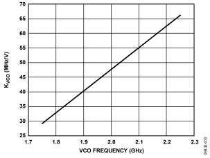
Figure 6. K<sub>VCO</sub> vs. VCO Frequency
