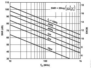
Figure 52. SNR and ENOB vs. Analog Input Frequency
