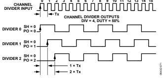
Figure 40. Effect of Coarse Phase Offset (or Delay)
