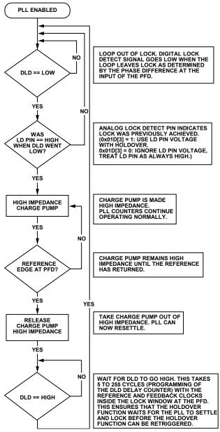
Figure 38. Flow Chart of Automatic/Internal Holdover Mode
