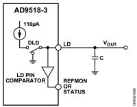
Figure 36. Current Source Digital Lock Detect
