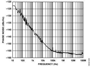
Figure 20. Phase Noise (Additive) LVPECL at 245.76 MHz, Divide-by-1
