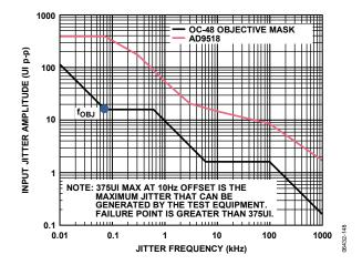
Figure 26. GR-253 Jitter Tolerance Plot
