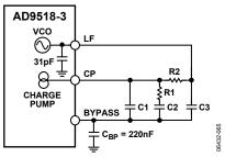
Figure 32. Example of External Loop Filter for a PLL Using the Internal VCO
