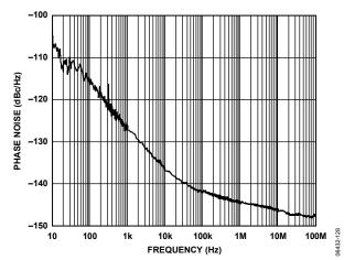
Figure 22. Phase Noise (Additive) LVPECL at 1600 MHz, Divide-by-1
