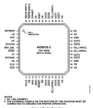
Figure 4. Pin Configuration
