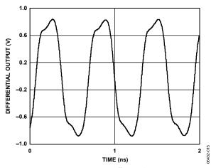
Figure 15. LVPECL Output (Differential) at 1600 MHz
