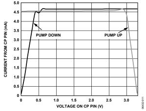
Figure 7. Charge Pump Characteristics at  $V_{CP} = 3.3 \text{ V}$
