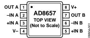
Figure 1. AD8657 Pin Configuration, 8-Lead MSOP
