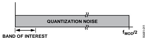
Figure 57. \Sigma - \Delta ADC Quantization Noise (Linear Scale X-Axis)
